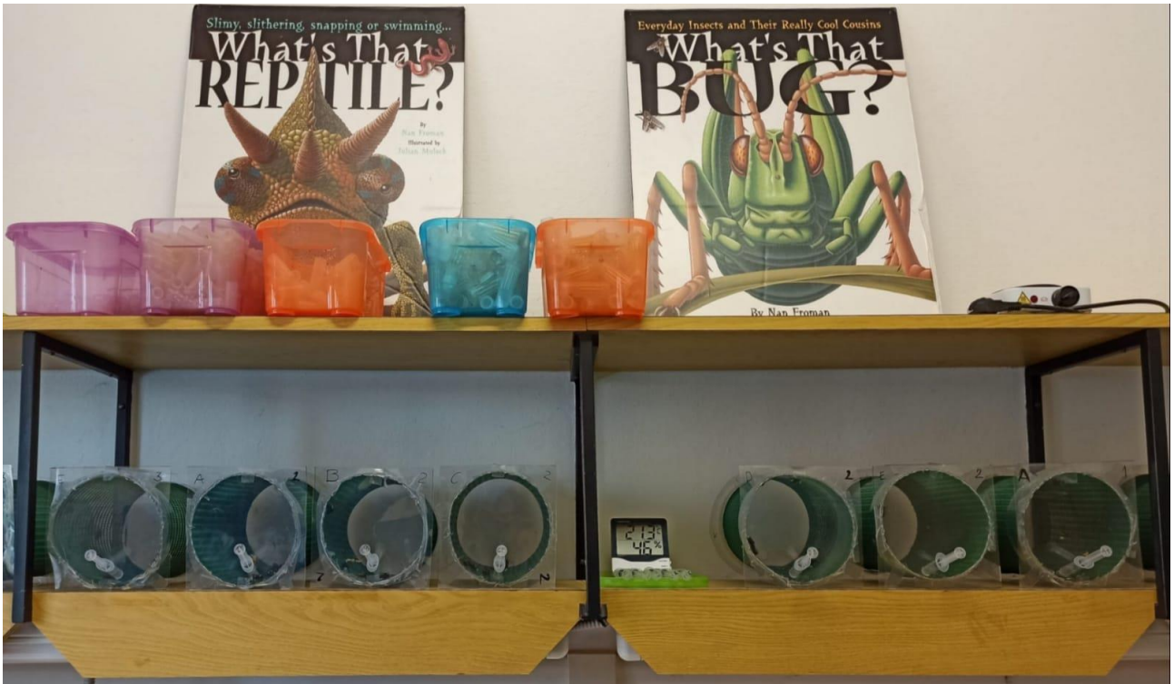
Figure S1. Flight cages used for the experiment on locomotion ( Exp. 2 ) consisted of plastic net cylinders (length = 25 cm, diam. = 16 cm) mounted horizontally with the ends closed by transparent plastic lids.
